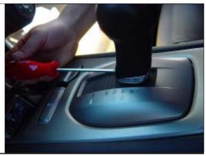
STEP 4. Pull the shifter knob off of the shifter shaft.
