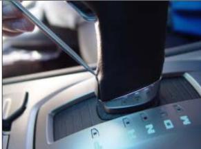
**STEP 3.** Unscrew the locking screw that holds the shifter knob onto the shifter shaft.
