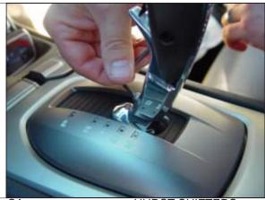
STEP 8. With the key in the ignition (vehicle "OFF") and foot firmly depressing the brake pedal. Cycle the shifter through all position to ensure smooth and accurate movement. If binding or rough movement occurs, review and ensure that all assembly steps have been completed as indicated.
